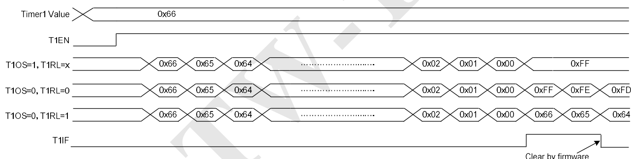
Figure 14 Timer1 Timing Chart
